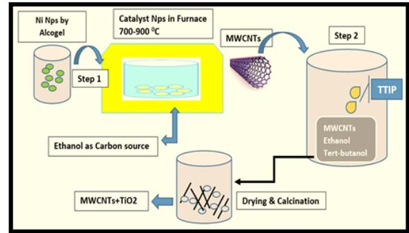
FIG. 1: Schematics for the preparation of  $\text{TiO}_2$  – MWCNTs nanocomposite.
