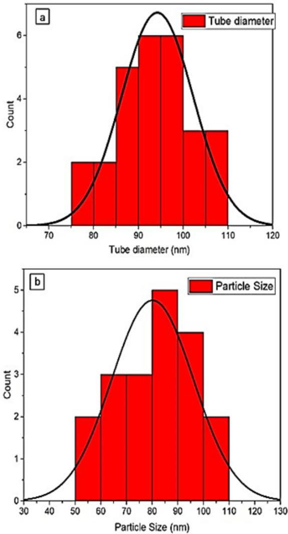
FIG. 3: The tube diameter and particle size distribution for MWCNTs and TiO<sub>2</sub>NPs<sup>2</sup> in TiO<sub>2</sub>-MWCNTs.
