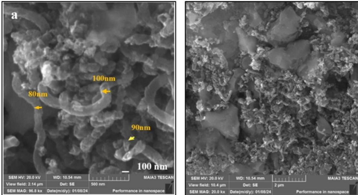
FIG. 2: FE-SEM images of the grown MWCNTs through CVD 500 nm (a) and at 2  $\mu$  m (b)
