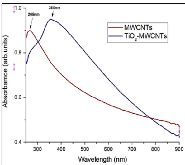
FIG. 6: UV-Visible spectrum for TiO<sub>2</sub> and TiO<sub>2</sub>-MWCNTs.
