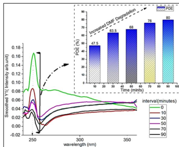
FIG. 7: UV Absorption spectra and photodegradation efficiency for DMF with incorporated TiO<sub>2</sub>-MWCNTs.
