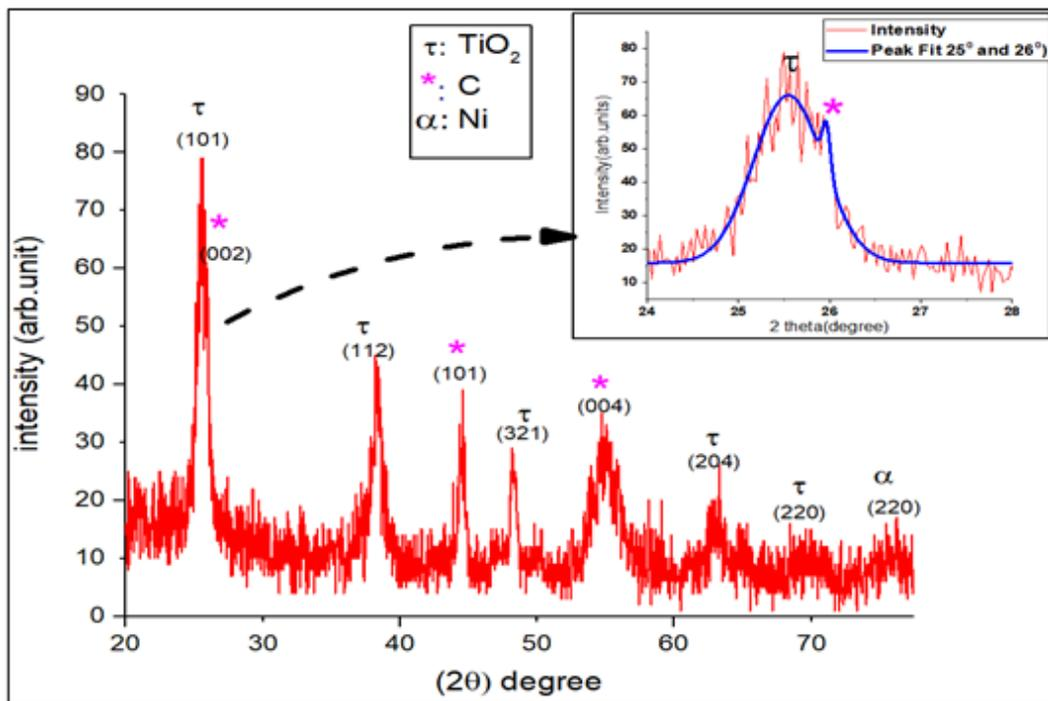
FIG. 5: XRD pattern for the prepared the TiO<sub>2</sub>-MWCNTs nanocomposite.
