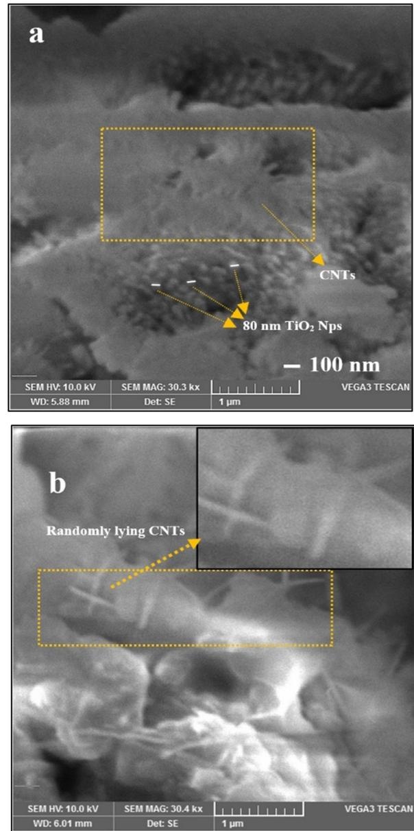
FIG. 4: SEM images of the TiO<sub>2</sub>-MWCNTs nanocomposite.
