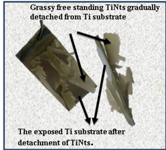
FIG. 2: The grassy free standing TiNts during detachment from Ti Substrate.
